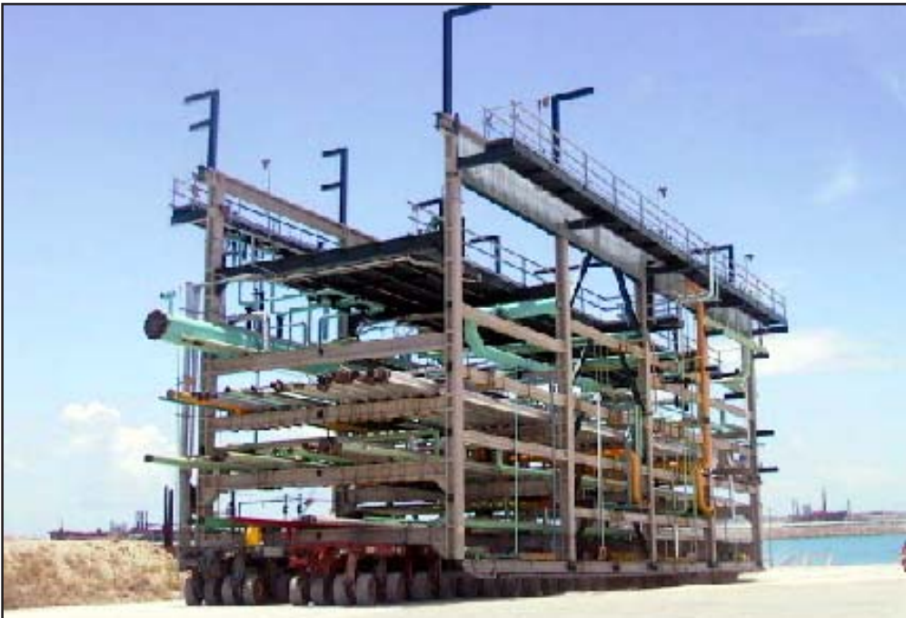
Figure 7.1-11 KAMAG Self-Propelled Transporters Hauling Module
